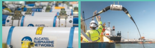
Clockwise from top: workers making cables in the 1800s; a repeater about to be deployed in the water; a number of ASN repeaters – these repeat the data signals along the length of the cables
